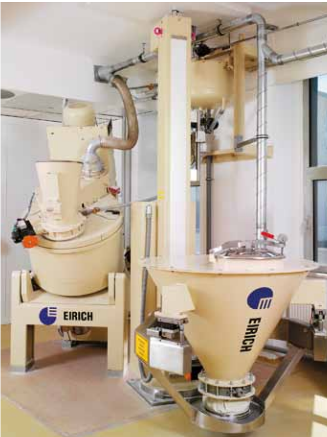
Scale assembly Additive storage and feeding Mixer with Quicklift feeding unit Mixer operator panel with touch display
